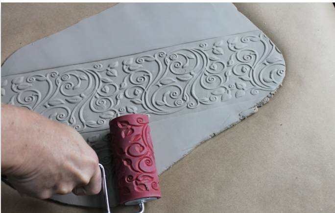
2. Apply texture. Press texture into slab using a texture roller, stamps, or press slab into texture molds.
