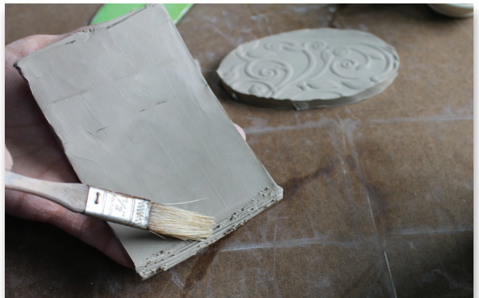
5. Paint on small amount of vinegar (used instead of slip for the glue) on scored places and attach.
