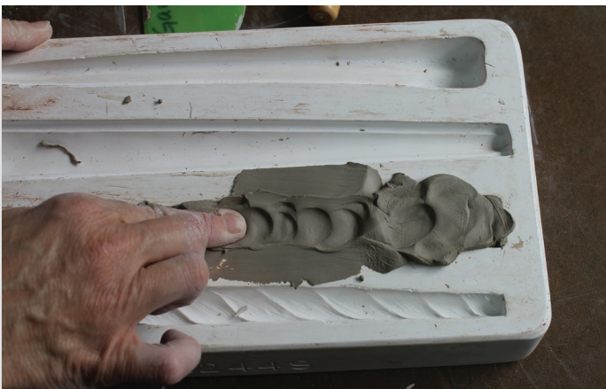
14. Press the amount of clay needed into the handle sprig mold. Press and repress clay into mold.
